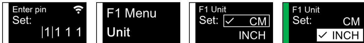
Figure 6: After specifying the correct pin, the menu opens (example of the unit settings)
