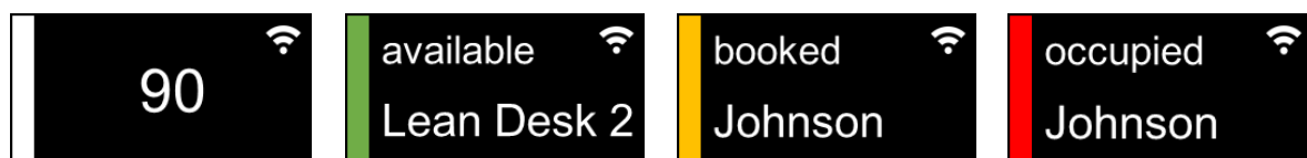
Figure 5: The controller can display different booking statuses and LED colors
