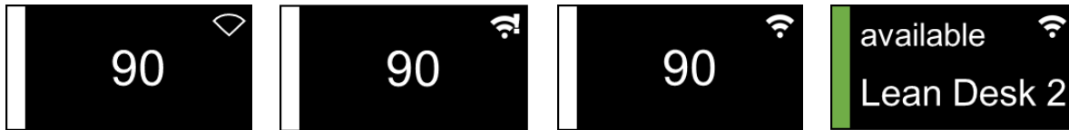
Figure 4: The WLAN symbol shows the communication status
